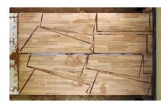
Nesting and plate optimization tools save time and materials, which can lead to an enormous increase in efficiency and reduction of costs.
